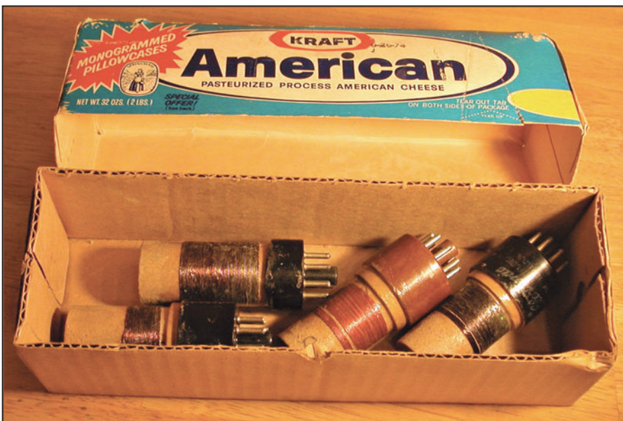
Photo I. Here's a close-up of our coil-winding skills. Pop and I weren't stingy when it came to putting on the Duco® cement! The enamel was scraped from the No. 22 wire, and the coil's leads for the top, bottom, and cathode tap were carefully pushed into the proper pin on the tube base. We were very careful in doing this work, because one mistake could result in having to start all over . It usually took a full evening to make one from start to finish. We got better at the process with each new plug-in we made.
