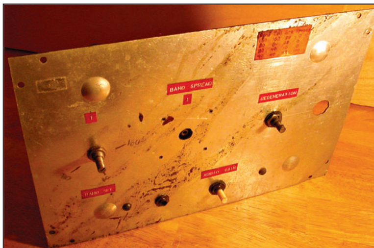
Photo A. It is clear to see that our "Little Electrical Disaster Survivor" has succumbed to time, scavenge, and the perils of Pop's radio sanctum since it was built six years ago. In happier times, the front panel was a thing of regenerative beauty with the band-set capacitor control on the left. In the middle, you can see the four holes where a nice vernier drive was mounted for band-spread tuning. The regeneration control was at the right and audio at the bottom. To the left of the audio was the headphone jack and the gaping hole on the upper right was where Pop and I put a pilot light — to remind me not to reach behind the front panel when the power was on. We made a little chart of capacitor settings and glued it near the top of the panel for easy reference. I'm not sure what that gunk is that dripped down the regen's face. It could be just about anything, given the rather "untamed" condition Pop's radio workshop was in. (Photography courtesy of KPC6KPH)
