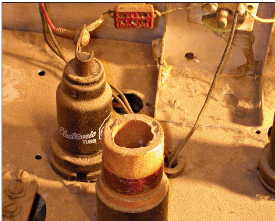
Photo G. Beneath the dust on top of the 6J7 Electronic Tube you can see the cap for its grid. That was a feature Pop really loved about this popular tube. We bent a Fahnestock clip just right to serve as our tube cap < http://bit.ly/1cvVw7F >. From the cap, there's a silver-mica "condenser" and a resistor going to the band spread tuning capacitor, "per our schematic," as Pop loved to say. By the way, that's the 7-MHz coil in the foreground.
